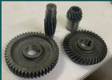
Paddle Wheel Aerators Gearbox
